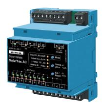
The SolarYes monitors outputs of inverters in PV-systems. Its output-relays (2 potential-free contacts) switch, when there has been no current during the last 24 hours in one of up to 8 monitored lines. Thus the failure of an inverter or a fuse is detected and reported. The operator can initiate repair immediately and saves downtime.
