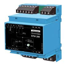
Current-relays STW200 monitor AC-currents for falling below an adjusted limit. The ranges 12 ... 120 mA and 0,1 ... 1 A allow the monitoring of LED-Lamps as well as incandescent lamps in obstruction lights.
