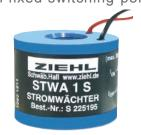
The STWA1S has an integrated electronic with transistor-output. The switching point is 2A. Above app. 2 A the output transistor is switched on (LOW), below app. 1.5 A it is off (HIGH).
