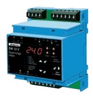
The voltage-relay SW12V is a high-grade device for monitoring DC- and AC-networks for overvoltage and/or undervoltage. 2 measuring-ranges 0...40,0 V and 0...300 V guarantee a high resolution.
