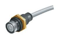
The light-sensor LF5 can be connected to the twilight-switches DS6 and DS 6V. It is mounted in a hermetically sealed, weather-proof and uv-resistant plastic threadid pipe. The connection-cable is 1 m long.
