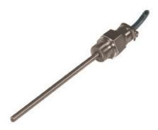
Platinum resistance temperature sensor built into steel tube V4A, 1/2 inch, suitable for installation in pipes. Thermal response time  $T_{\rm 0,9}$  in the air 255 s, in water 45 s.
