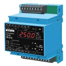
The limit value switch TR210 monitors up to 2 measuring inputs for Pt100 (RTD), Pt1000, thermocouples, or standard-signals 0/4-20 mA, 0-10 V.
