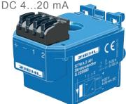
The STWA2AH is a measuring transducer for AC currents 0...100 A, divided in 2 ranges 0...20 A and 0...100 A. Multiple loops of the conductor through the transformer reduces the measuring range correspondingly (for instance to 0...5 A with four loops).
