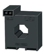
The ASS500/5 plug-in-current-voltage transformer is a measuring transformer with high linearity for currents up to AC 500 A and an output signal of 5 mV per ampere. Its maximum error is 1% of the measured value. The instrument is simply plugged onto the current-carrying conductor.
