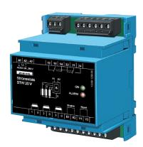
The current relay STW20V monitors the current in up to 3 lines with current transformers STWA 1 (AND circuit). If there is a current in all 3 monitored lines, the relay (2 change-over contacts) picks up. If there is no current in at least one of the lines, the relay releases.
