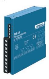
The level monitor NS43 regulates the level of liquid in a container between 2 electrodes. In the normal operation the level of the liquid is situated between the electrodes E2 and E3. The relay K2 tightens, if the level E3 is achieved and drops, if E2 is fallen below. Over the output contacts (1 change-over switch) a pump or a valve can be controlled depending upon case of application and so the level be
