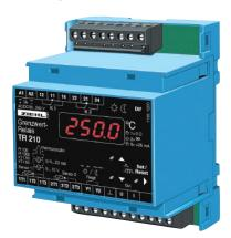
The limit value switch TR210 monitors up to 2 measuring inputs for Pt100 (RTD), Pt1000, thermocouples, or standard-signals 0/4-20 mA, 0-10 V.
