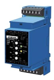
ZIEHL STW1000V2 current relays monitor standard signals from instrument transformers for compliance with a limit value. Units can be wired in series (current) or in parallel (voltage) to monitor multiple limits.
