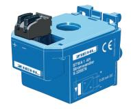
The STWA1AH is a measuring transducer for AC currents 0...15 A. Multiple loops of the conductor through the transformer reduces the measuring range correspondingly (for instance to 0...5 A with three loops).
