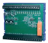
The current relay STW12 monitors the current flow yes/no of up to 12 alternating-current circuits. If there is an AC-current of ≥1 A through a connected transformer STWA 1, the according output transistor switches and the yellow LED lights up.
