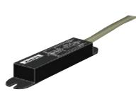
The current sensor S1 records the current in a cable with a hall-sensor. At currents of app. 5 A (adjustable version 5-30 A) the transistor-outputs switch and report a current in the monitored cable.
