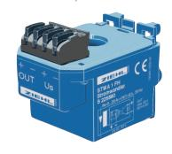
The STWA1FH provides a frequency output with 0.5...20 Hz which corresponds to a current flow of AC 0 - 20 A through the transformer. Multiple loops of the conductor through the transformer reduce the current range correspondingly (e.g. with fourfold looping-through 0 - 5 A correspond to 0.5...20 Hz).
