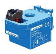
Current-transformers STWA1H can be fixed on a 35 mm DIN-rail or with 2 screws.
